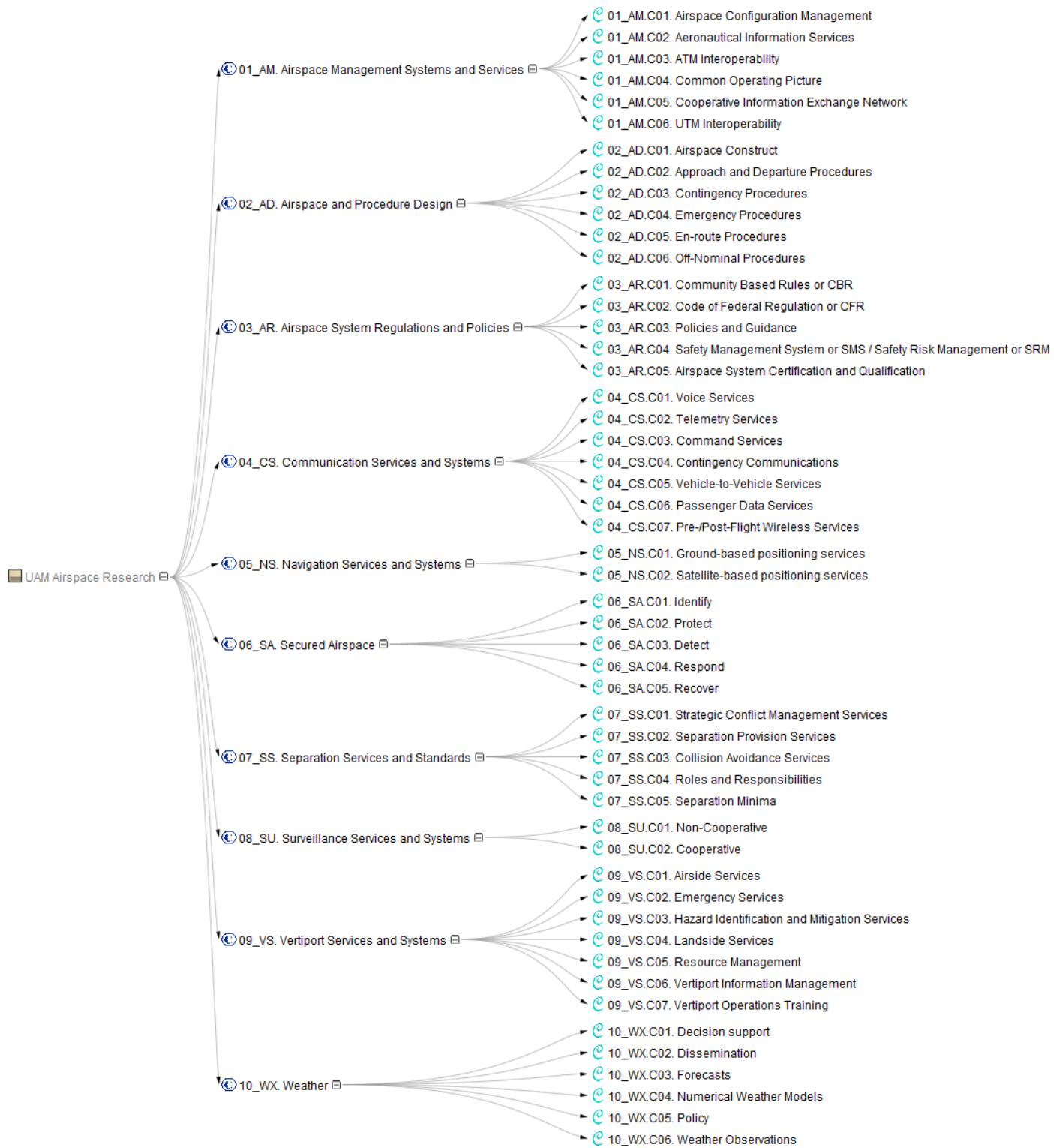
Figure 1. UAM Airspace Capability and Component Tree Decomposition
