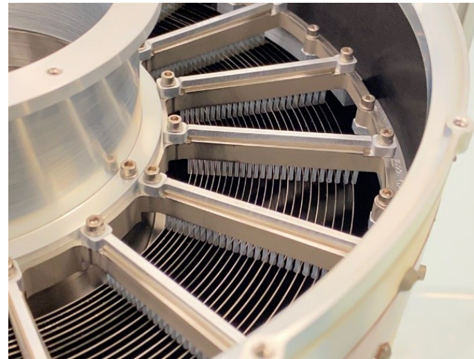
Rear of MMA Showing 24 Nested Mirror Shells
