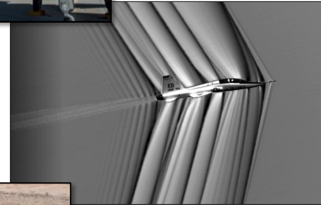
Advanced Air-Air Schlieren Imaging
