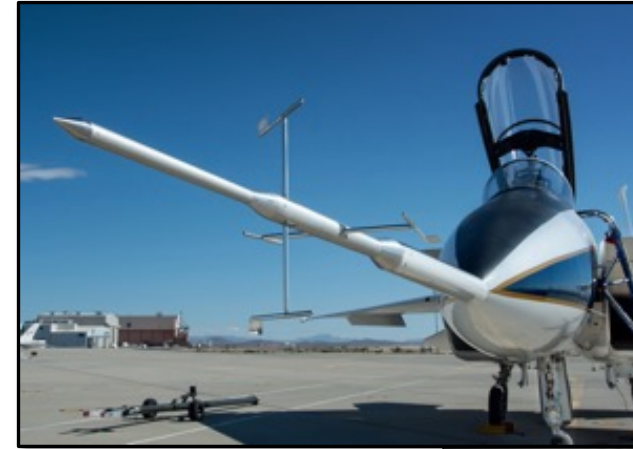
F-15 With Shock Sensing Probe
