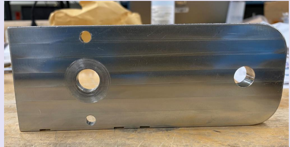
Coupon visibly clean, 3.78mg NVR collected
