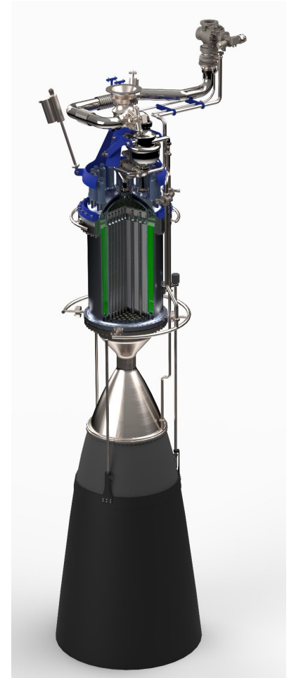
NASA's NTP Engine System is shown, of which BWXT is providing support for reactor and fuel design and analysis and AR is providing support for engine component design, analysis, and integration.(25,000 lb f )
