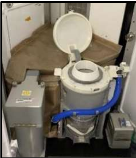
ISS UWMS Trainer at JSC with Acoustic Cover
