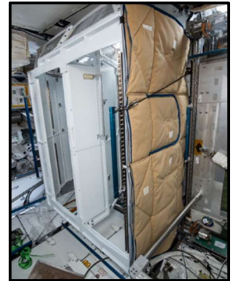
ISS UWMS and Toilet Stall in Node 3
