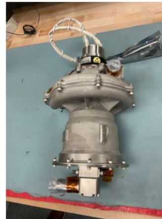
ISS UWMS Dual Fan Separator (top images and left lower image) and attempt to move stuck separator with on-orbit vacuum cleaner (right lower image)
