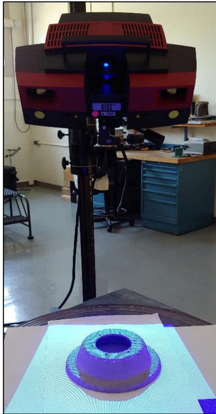
ATOS structured light scanning unit projecting fringe pattern on to part
