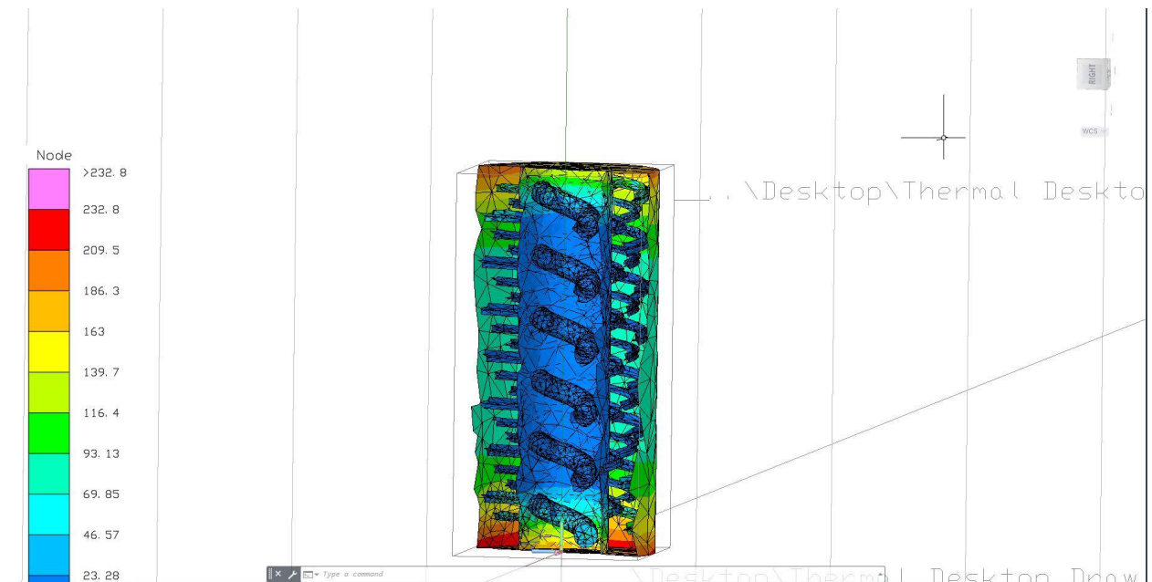
Figure 4.11. Cooling using negative wattage on heater.
