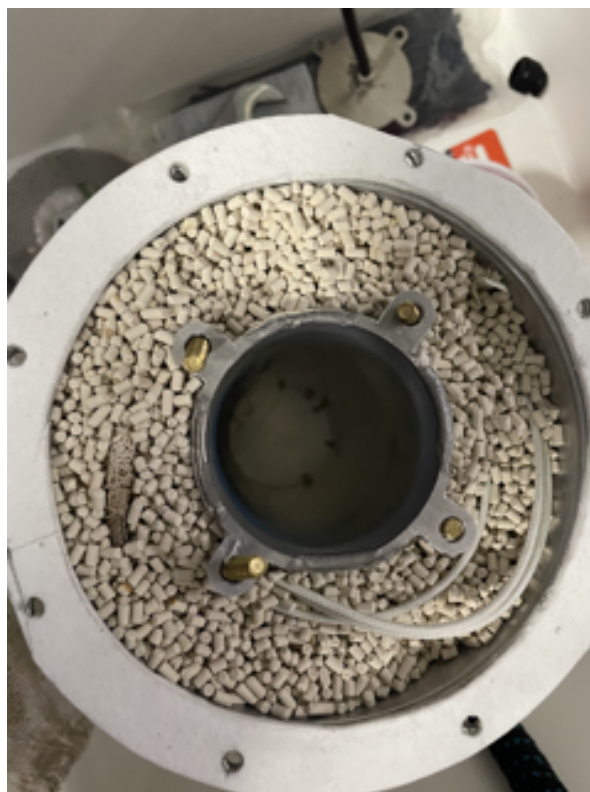
Figure 6.3. Inside bed with heat tape and zeolite
