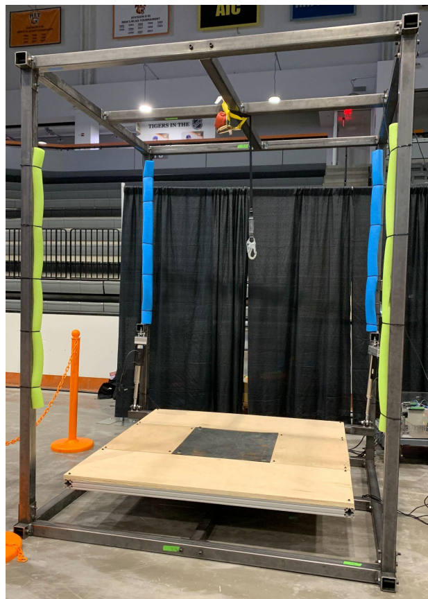
Figure 2 - shows the assembled rig and motion floor with attached anchor point and retractable harness strap.
