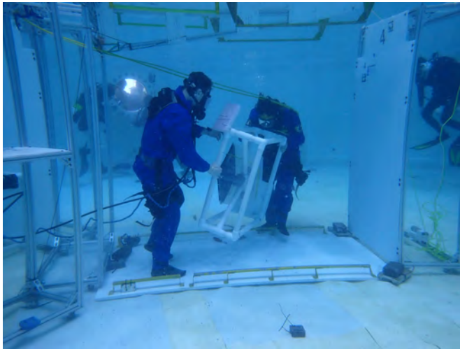
Figure 125: Images from the lunar test. Divers are moving the equipment out of the simulated core to the securing site, representing the first step in the testing procedure.
