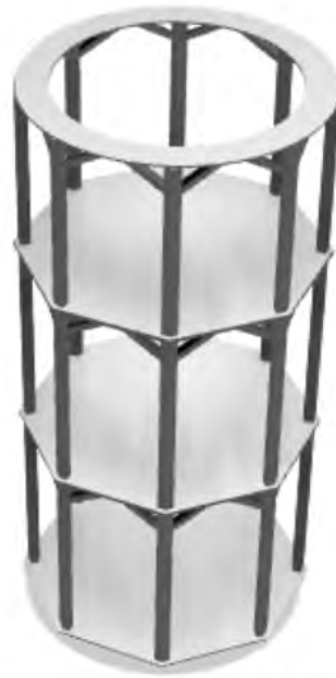
Figure 35: The final iteration of the core design with octagonal floors, more diagonal support members, and vertical supports meant to accommodate structural trusses
