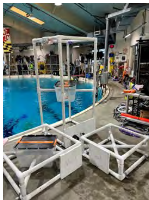
Figure 120: Test equipment used for micro-g and lunar tests. The small, medium, and large PVC structures are displayed.
