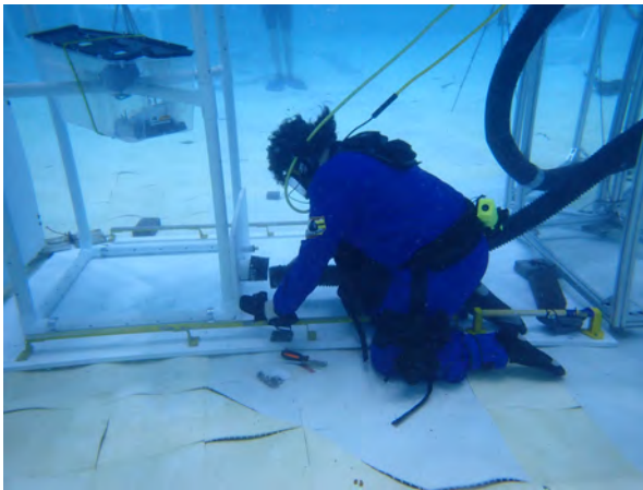
Figure 127: Images from the lunar test. Diver is attaching utility lines to the equipment, representing the third step in the testing procedure.
