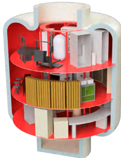
Figure 156: The uniformly illuminated surfaces in the habitat for the first analysis, represented in red.
