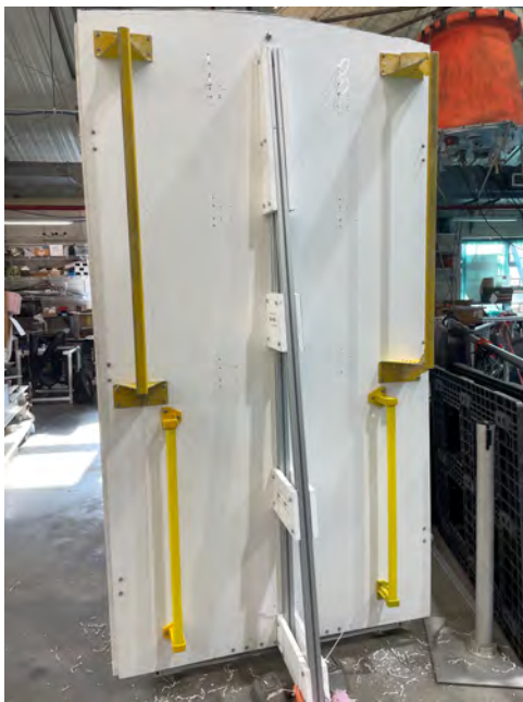
Figure 84: Images of handles and weights added to the floor panel in preparation for the second dive. The image on the right shows the testing rig being lowered into place after being properly weighted.
