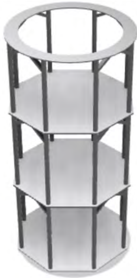
Figure 30: The second iteration of the core design with octagonal floors and support members to limit lateral deflection
