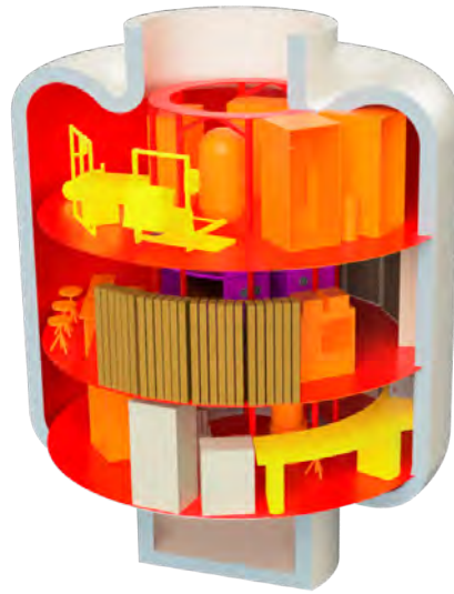
Figure 158: The illuminated surfaces in the habitat for the third analysis with color representing illumination level. Purple is a sleep illumination or 54 lux, red represents a general illumination of 108 lux, orange and illumination of 269 lux, and yellow an illumination of 323 lux.
