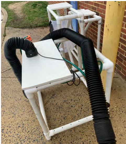
Figure 145: Images of the setup for 1g equipment testing. The secondary structure housing the lines (left) and the large PVC structure with lines connected and secured (right).
