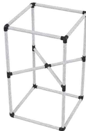
Figure 119: PVC test equipment designed for micro-g and lunar tests. Joint parts are colored in black.
