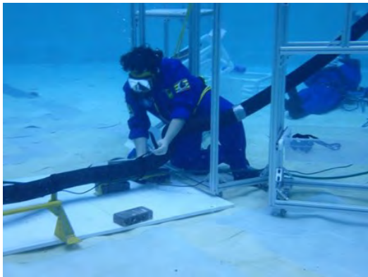
Figure 124: Images from the micro-g test. Diver is attaching utility lines to the equipment, representing the third step in the testing procedure.
