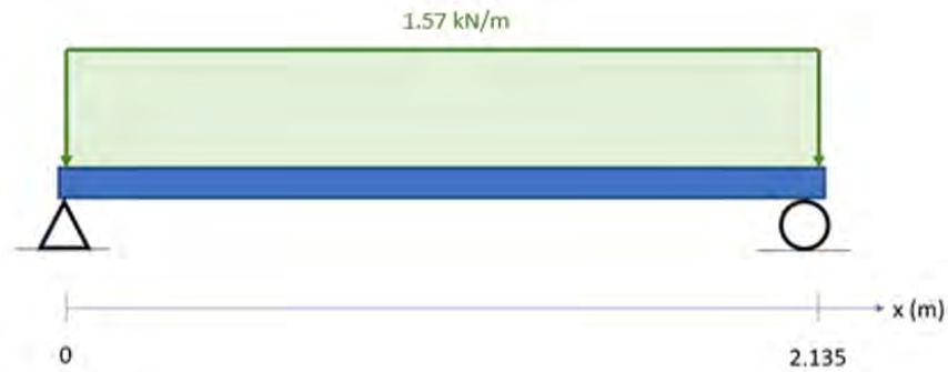
Figure 55: Initial support beam with rectangular distributed load and with pinned connection at core (left) and roller support on inflatable structure (right)
