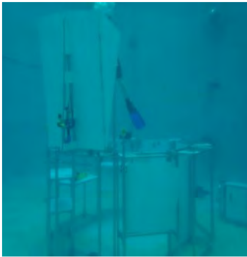
Figure 79: Images from the April 8 test of the floor panel deployment. The left image is the floor in its upright position and the right image is the deployed floor with the necessary weights on it.
