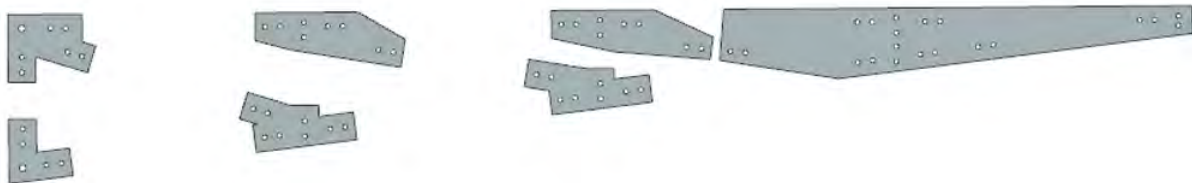
Figure 62: The design of the gusset plates relative to their location on the actual truss model
