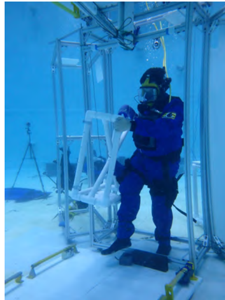
Figure 125: Images from the lunar test. Divers are moving the equipment out of the simulated core to the securing site, representing the first step in the testing procedure.
