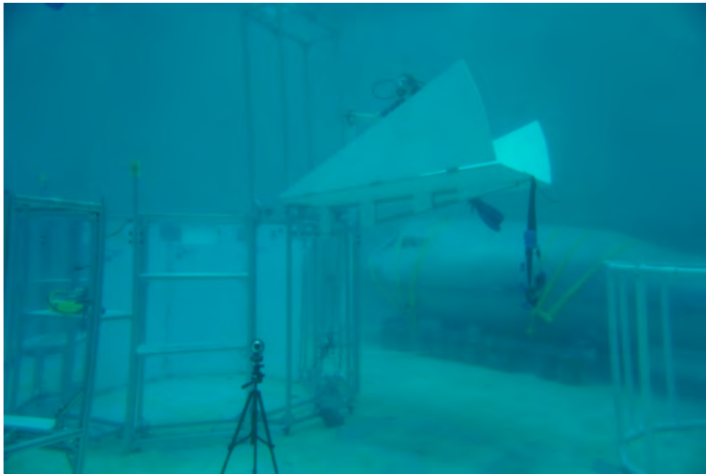
Figure 83: Image of first Neutral Buoyancy Tank dive for testing floor deployment.
