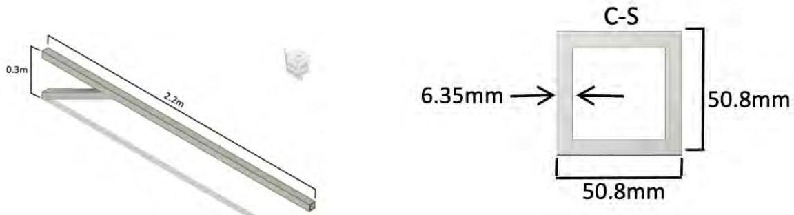
Figure 70: Micro-gravity floor support beam dimensions. Image on the right is the cross sectional dimensions of the beam. Image on the left is the length and height of the beam.
