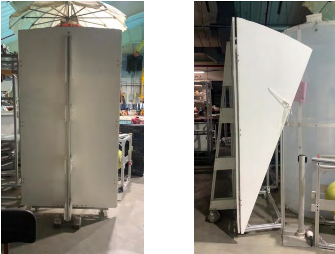
Figure 81: Images of the floor deployment test rig with a full scale floor panel attached.
