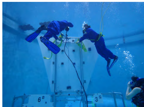
Figure 84: Images of handles and weights added to the floor panel in preparation for the second dive. The image on the right shows the testing rig being lowered into place after being properly weighted.
