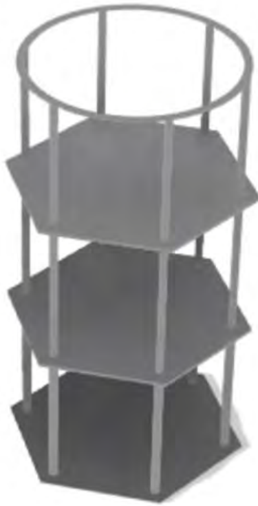
Figure 27: The first iteration of the core design with hexagonal floors and simplified construction
