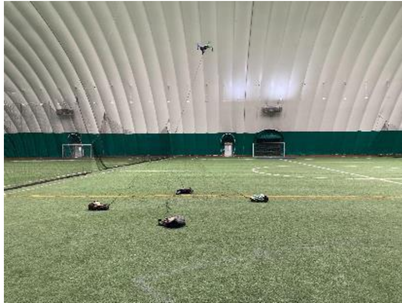
Figure 14: The drone is pulling on the netting material to check for any points of strain or bunching and so that we can verify the netting can withstand being pulled on by the drone.
