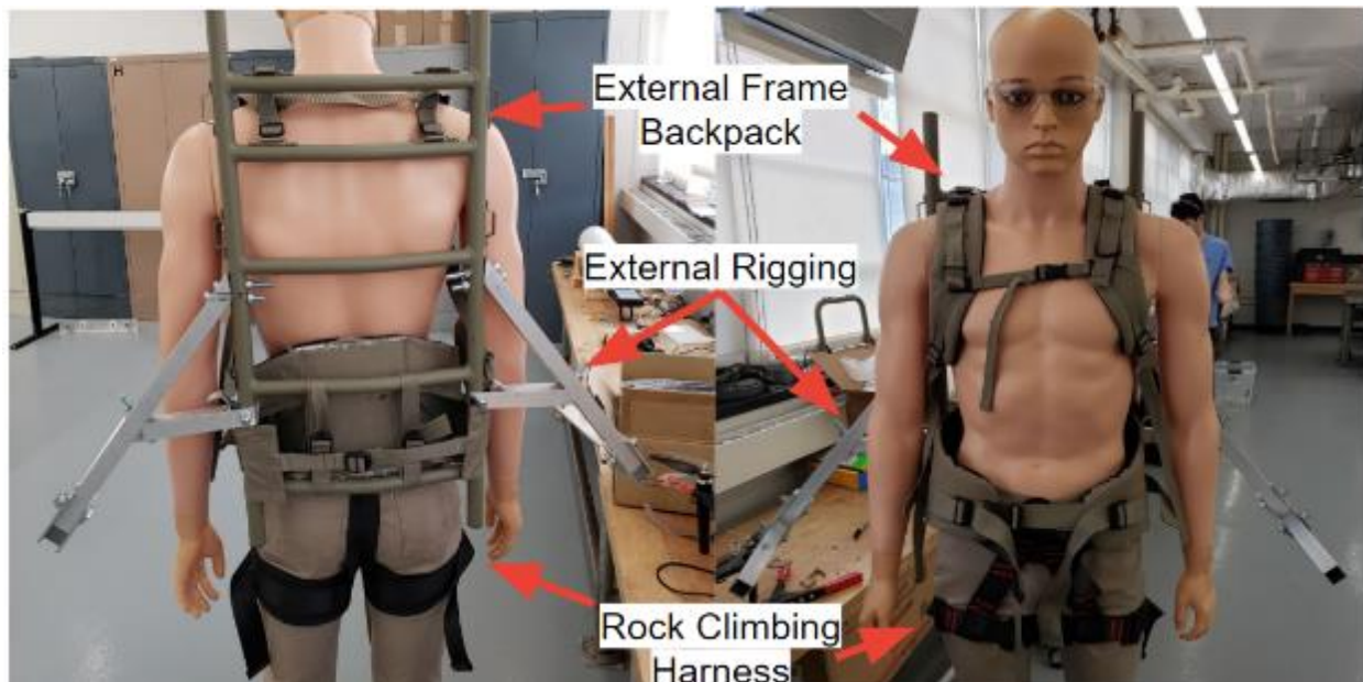
Figure 6: Gimbal system fitted to the mannequin.
