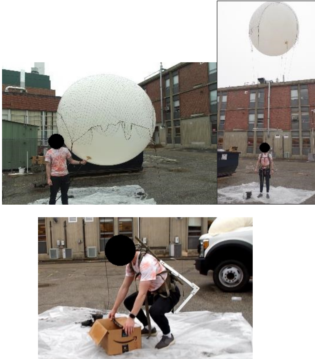
Figure 15: Shots from full scale testing that show filling up the balloon, a group member donning the suit and simulating picking up a box to show what an astronaut would endure during testing.
