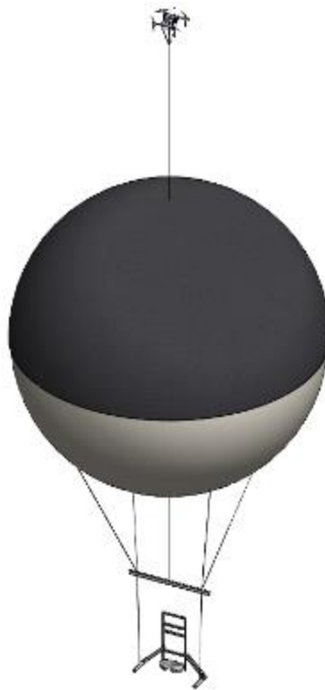
Figure 17: One Balloon Version: Balloon is 14ft diameter and is able to offload 100 lbf. Tether system would be identical and scaled up from our current system
