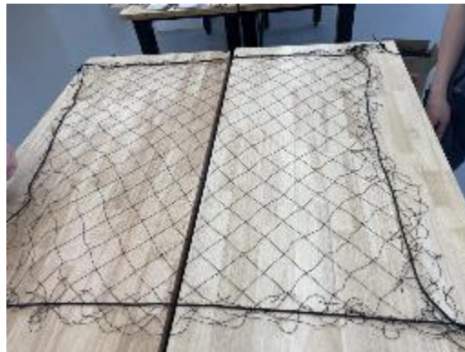
Figure 13: Small-scale version of netting with paracord edges and carabiner attachments then used to test initial load. The purpose of the small scale version was to prove the concept and plan fabrication before moving forward with a 10x10 ft version.
