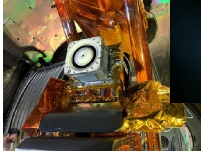
BHT-6000 thruster operating during 6kW EP string test at NASA GRC
