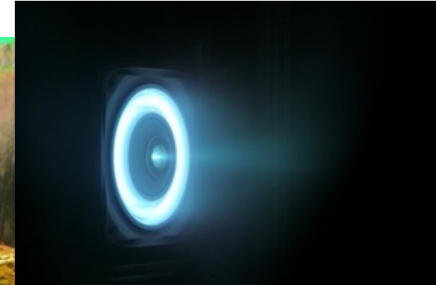
BHT-6000 thruster operating during 6kW EP string test at NASA GRC
