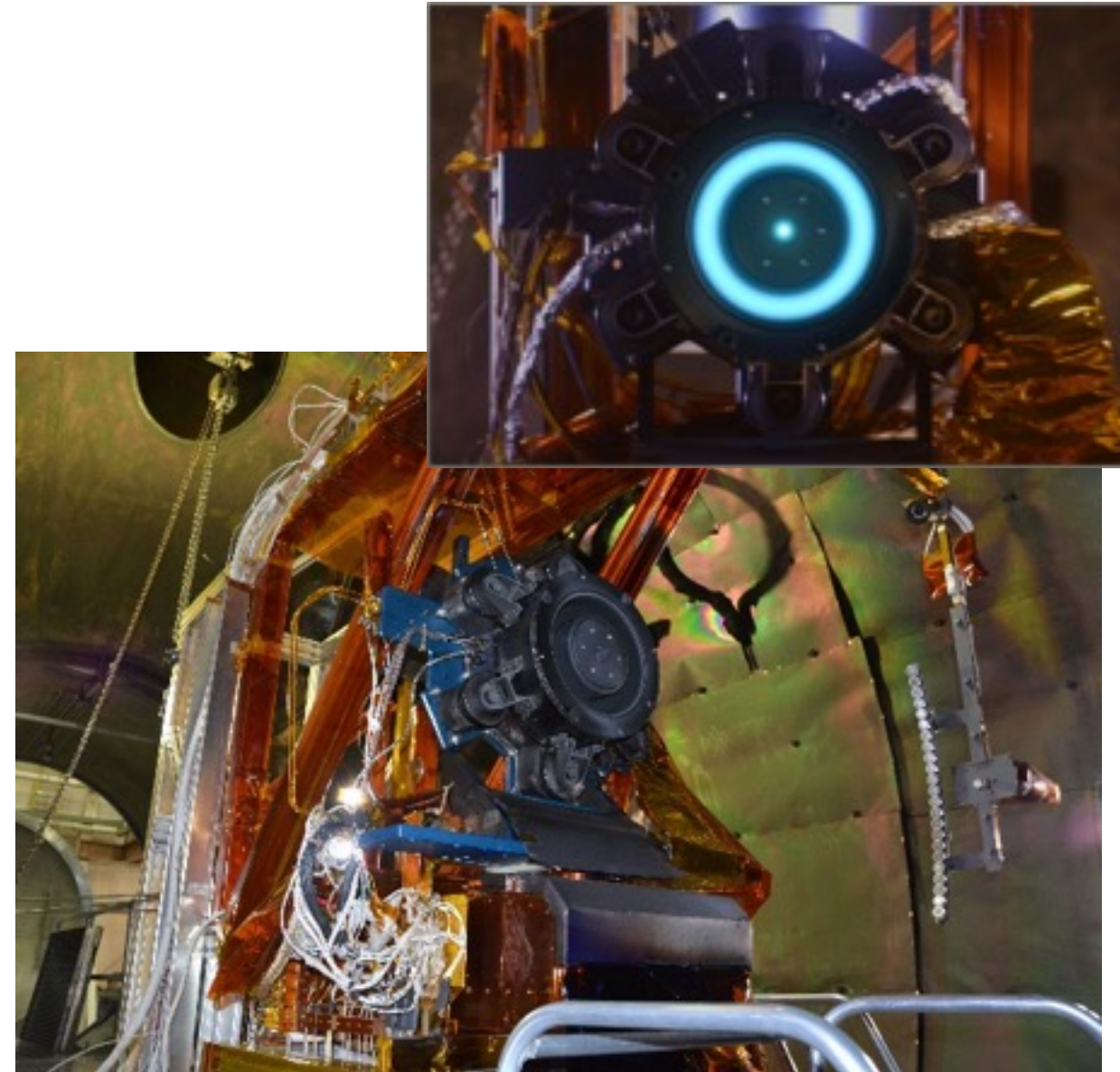
AEPS ETU-2 Thruster in NASA GRC VF-6 during 12kW Integrated String Testing.
