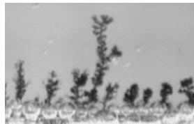
Dendrite growth in lithium metal batteries. Wood et al. ACS Central Science. (2016)
