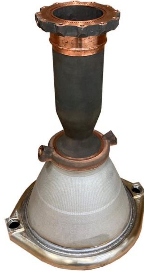
Direct deposit LP-DED nozzle (Axial Bimetallic)
