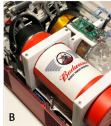
(A) 2U CubeLab growth chamber installation. (B) Malting CubeLab investigation with fluid and thermal control subsystems. (C) On-Orbit plant growth image.
