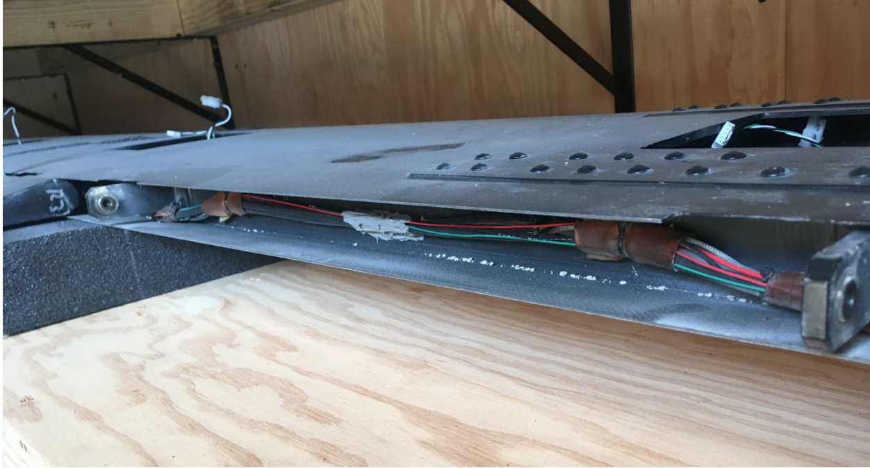
Figure 12. The X-56A MUTT hinge-gap pocket formed by wing skin extensions.
