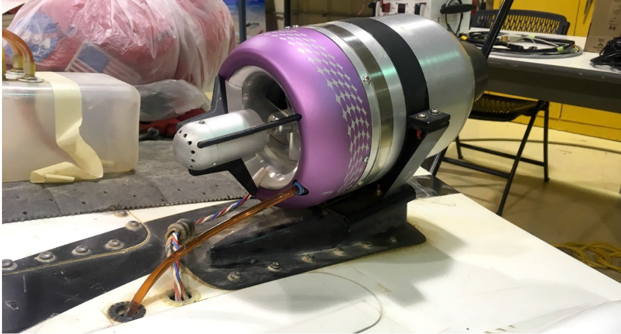
Figure 17. The X-56A Multi-Utility Technology Testbed JetCat P400 engine with starter generator in a podded (external) configuration.
