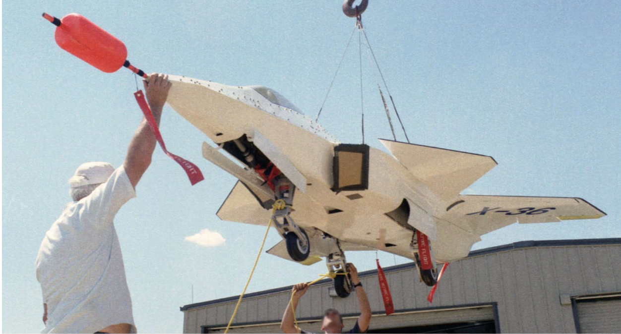
Figure 5. The X-36 Tailless Fighter Agility Research Aircraft being lifted by designed-in lifting points.
