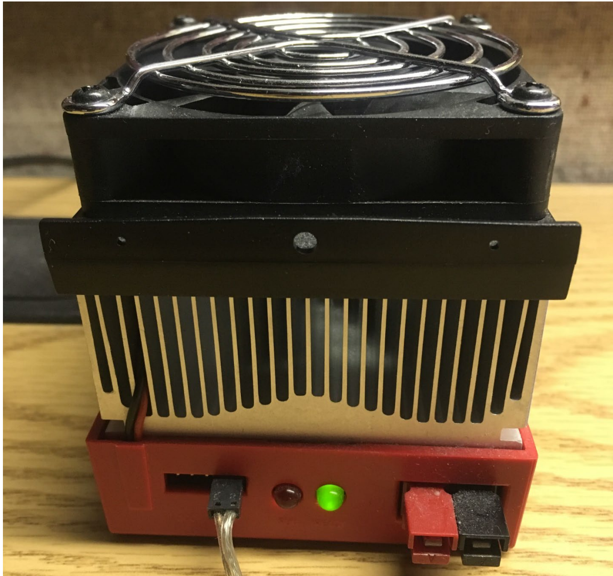
Figure 19. RF component-heat sink-muffin fan “sandwich.”
