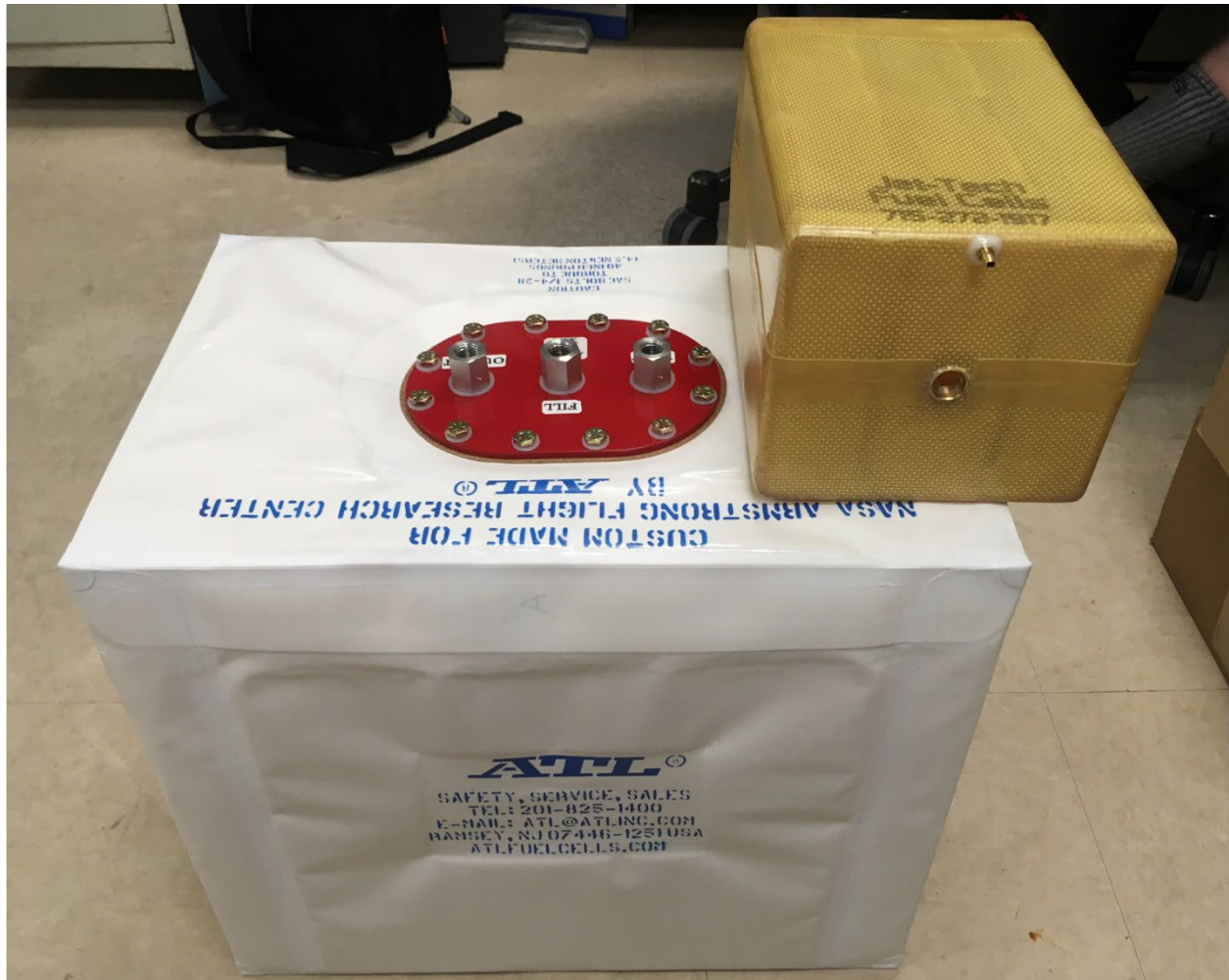
Figure 6. Rigid-walled (white) and flexible-walled (tan) bladder-type fuel tanks.
