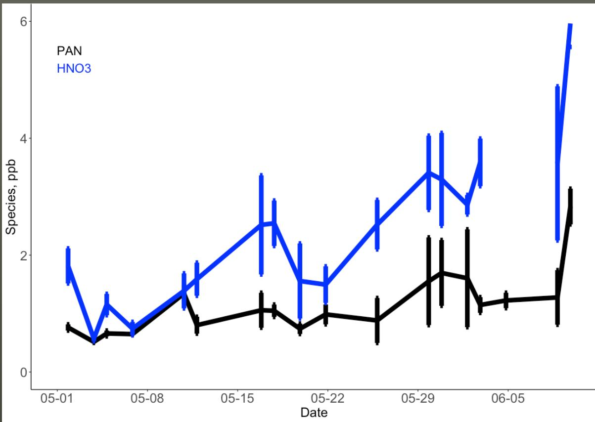
Figure S4. Average PAN and  $\text{HNO}_3$  below 0.5 km between 10 to 16 KST from the DC-8 aircraft descents described in Section S2. The PAN measurement is from the Georgia Tech chemical ionization mass spectrometer (GT-CIMS) and the  $\text{HNO}_3$  measurement is from the Caltech CIMS (CIT-ToF-CIMS).
