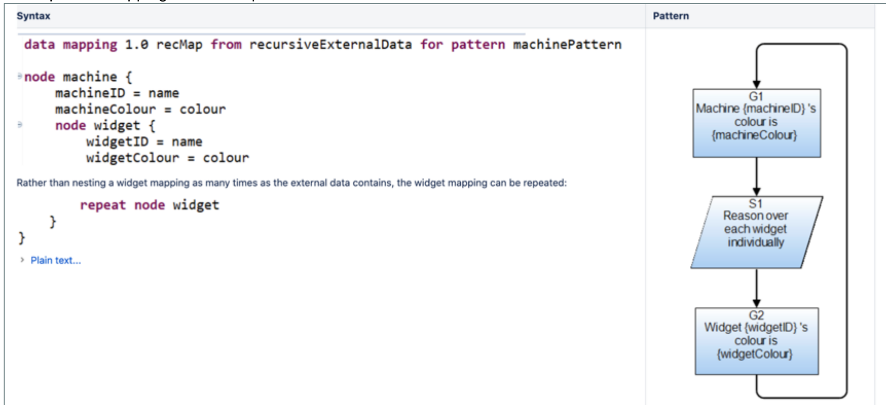
Figure 50: You can use the repeat node in a Data Mapping File for recursive reasoning in Argument Patterns (called Pattern Loops).
