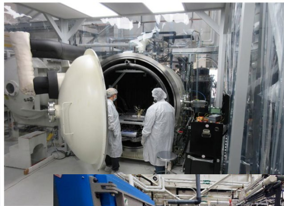
Chassis and Optical Head Thermal/Vacuum Test
