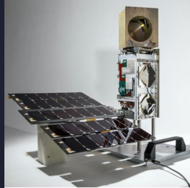
CubeSat/Nanosatellite TROPICS 3U/6U (1 – 10 kg)
