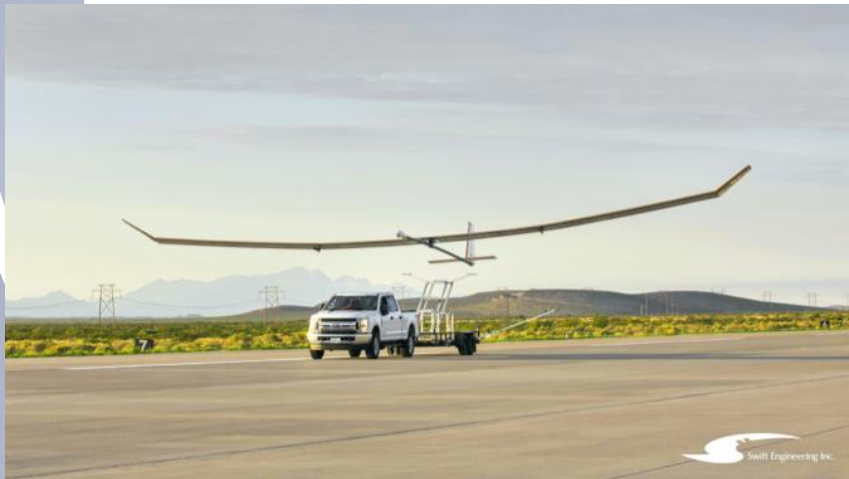
Swift Ultra Long Endurance UAS releasing from launch vehicle during first flight in July 2020 in New Mexico. The vehicle was designed to stay aloft for 30 days at 20km with a 5kg payload.
