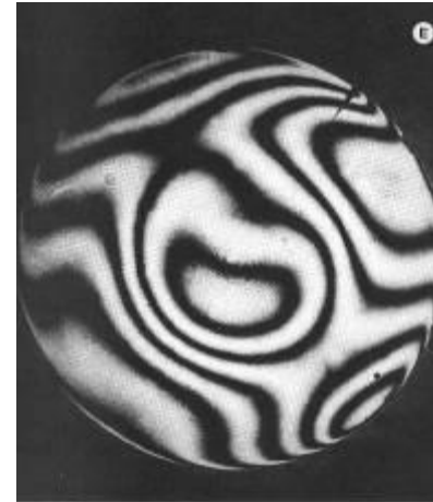
Thin Deformable Mirror - Before Active Optics System Activated
