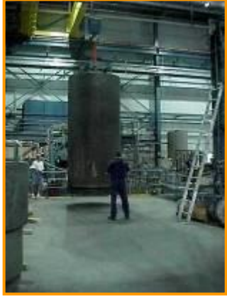
HIP Vessel being loading into chamber
