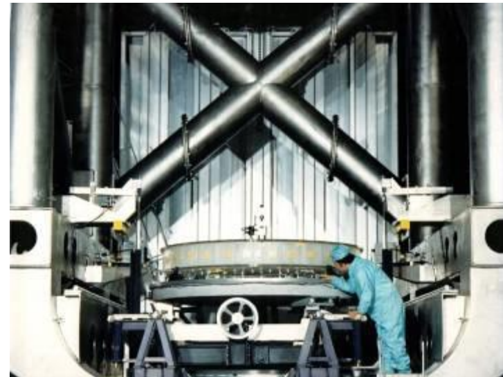
Start of Small Tool Computer Controlled Polishing
