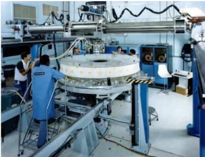
Start of Small Tool Computer Controlled Polishing
