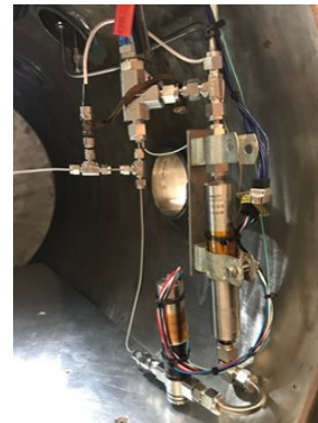
Figure 20: Incorporated Micro-Pump CubeSat Propellant System
