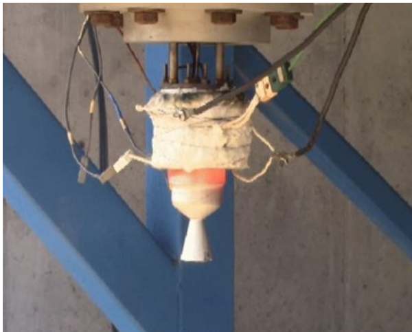
Figure 17: 100N Thruster during Hot Fire Test in Ambient Pressure
