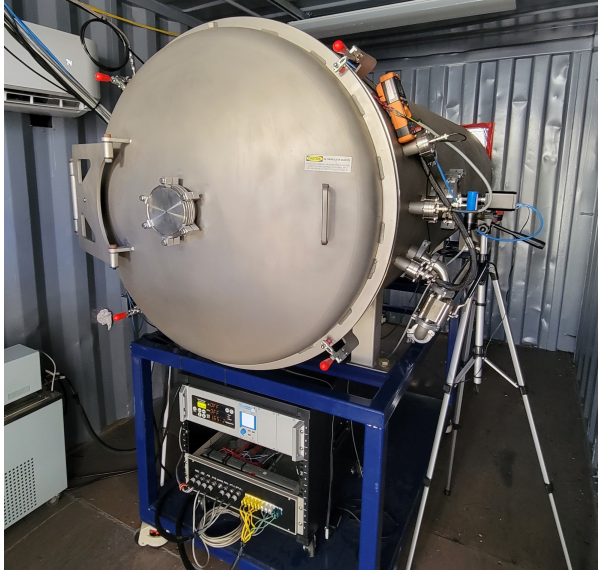
Figure 23: Hot Fire Test Vacuum Chamber
