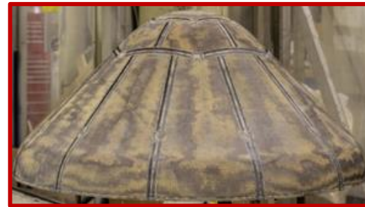
1.0-meter diameter tiled HEEET engineering test unit
