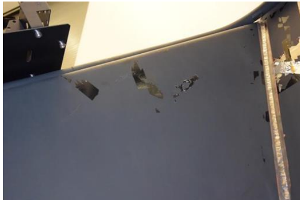
Figure 16. Tape backing completely delaminated from adhesive after exposure to cryogenic T in vacuum. (Photo credit: NASA/Joe Ward)
