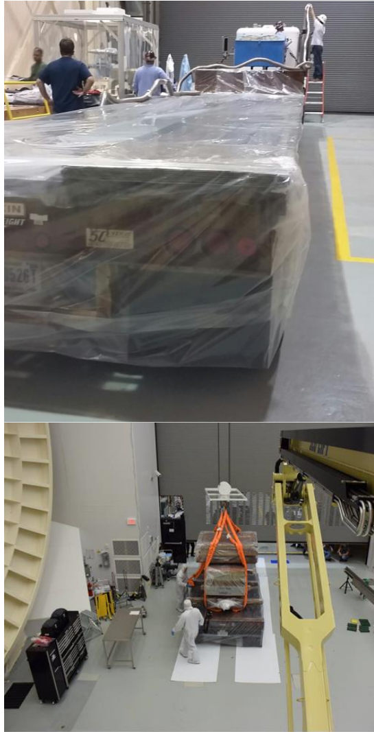
Figure 21. Truck trailer being prepared in truck lock then backed into cleanroom with crane load test weights ( Photo credit: NASA/Joe Ward, Chris Gunn )
