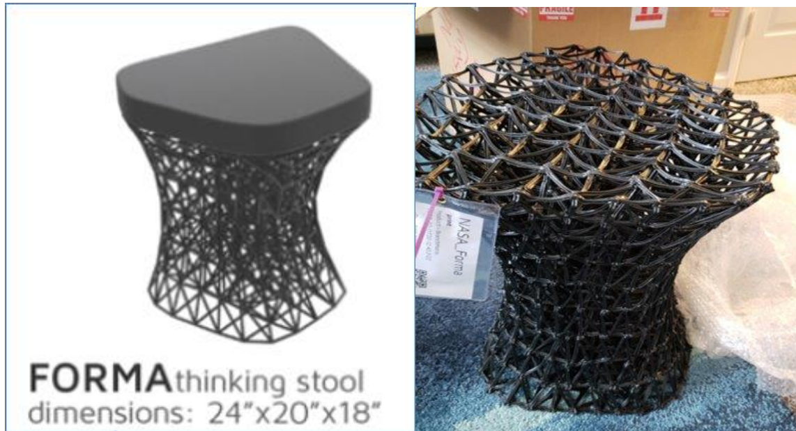
Figure 24: Design and photo of the test Forma stool printed by Branch Technology.
