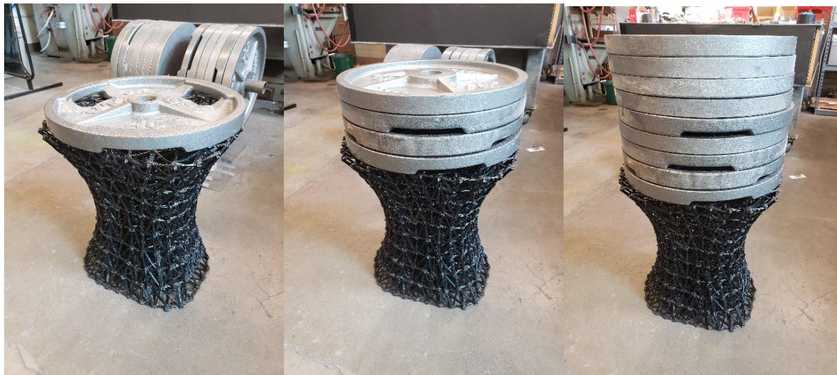
Figure 25: Loading testing of the test print stool at 20.4 kg (45 lbs), 81.6 kg (180 lbs), and 183.6 kg (405 lbs) from left to right respectively. Testing was stopped at 183 kg.
