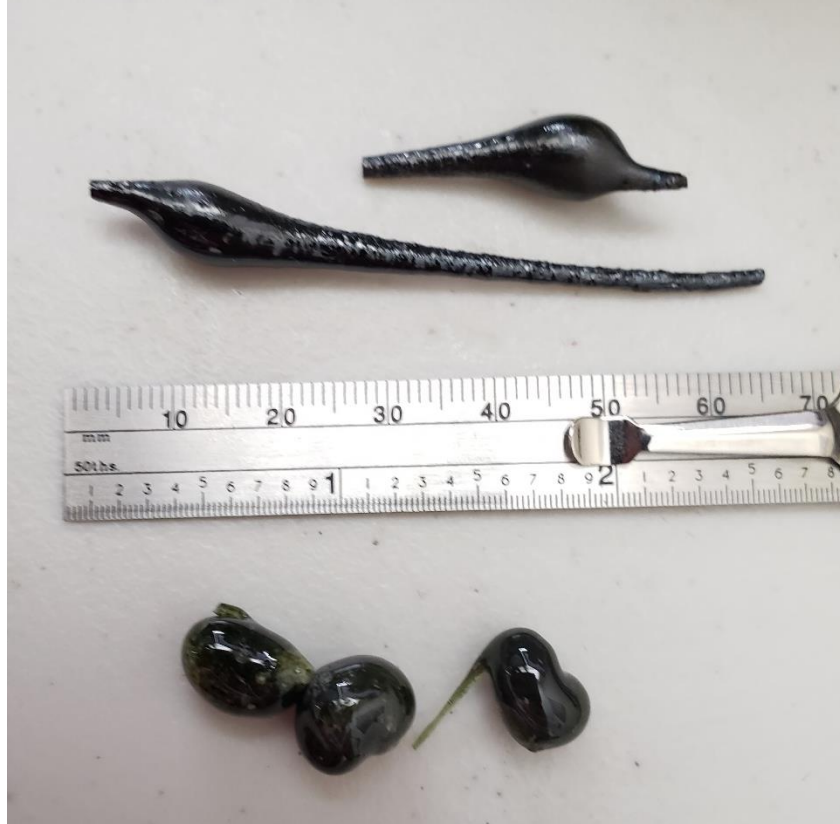
Figure 26: Example of the as-received vitrified simulant. JSC-1A material is shown at top, CSM-LHT-1 is shown below
