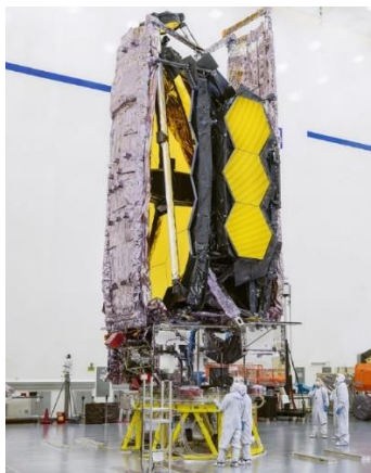
Figure 2. JWST Pre-Deployment Stowed Configuration 3
