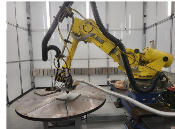
DM3D Directed Energy Deposition
