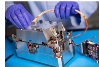
100 mN thrusters on Lunar Flashlight Propulsion System
