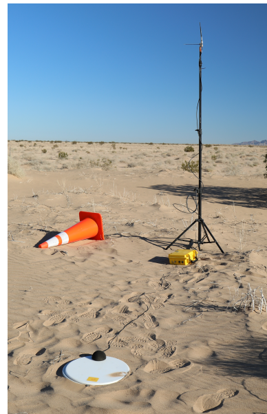
Fig. 2: WAMS II setup with GRAS 67AX microphone.
