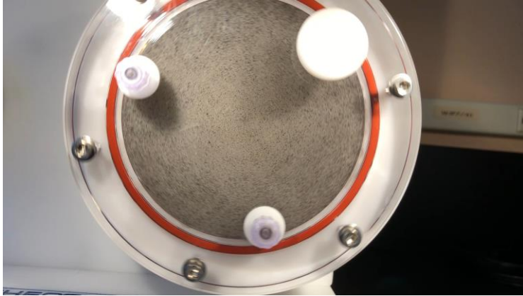
HARV with experimental flakes rotating at 15 rpm for particle tracking
