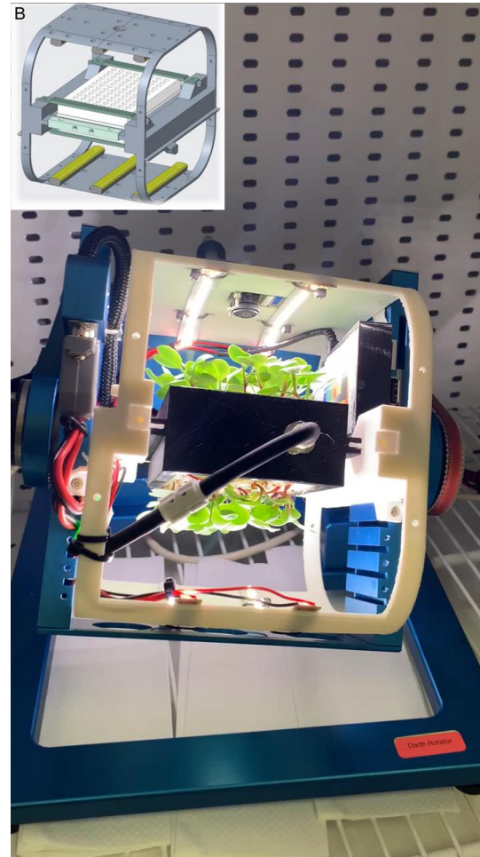
Plant growth chamber designed for microgreen study and other plant research
