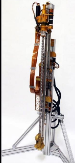
Subsurface excavation TRIDENT Drill
