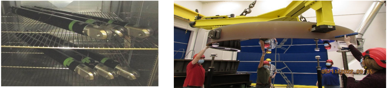
Figure 12. (a) FOA struts during thermal cycling (left) have also completed load testing. (b) Coated flat mirror for double-pass optical test of the telescope ready for final optical test before assembly for the thermal vacuum chamber.
