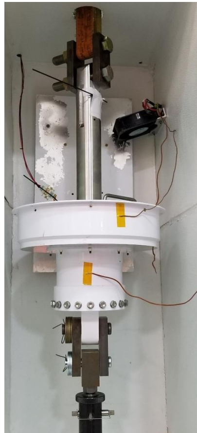
Figure 11: Thermocouples on the 5.5K Rotator
