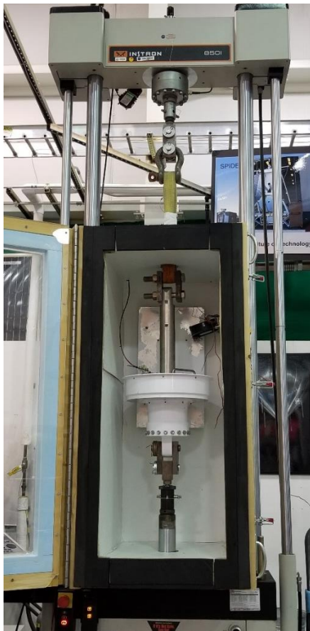
Figure 10: Thermal Test Setup in Instron Machine
