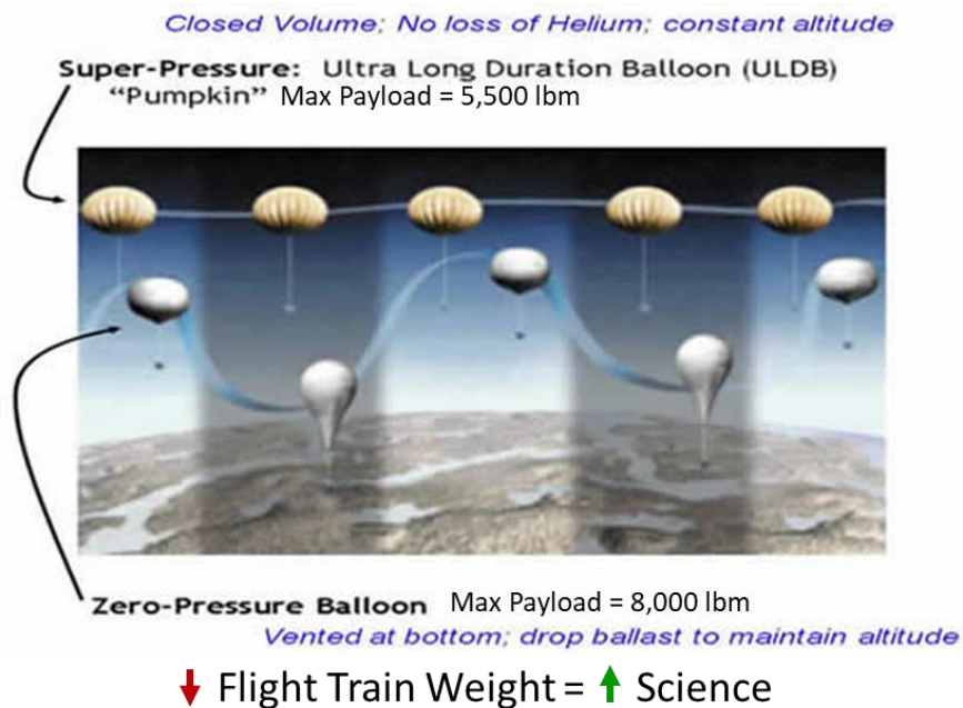
Figure 3: Super Pressure Balloon (SPB) vs. Zero-Pressure Balloon
