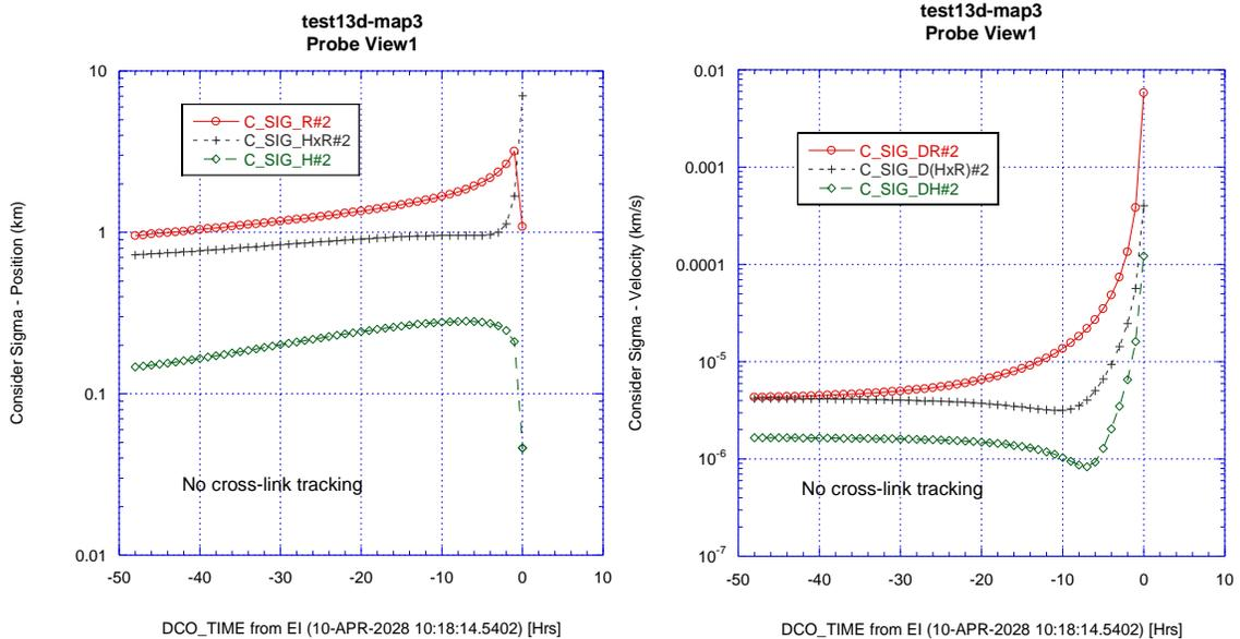
**Figure 2. Baseline Case: Position and velocity uncertainty (1- $\sigma$ ) of Probe from Probe Separation (EI-48h) to EI with no tracking. Venus-centered [R,HxR,H] coordinates.**
