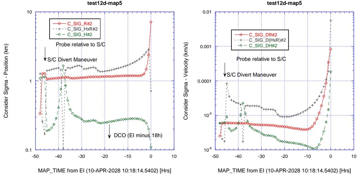
**Figure 4. Relative position and velocity uncertainty ( $1-\sigma$ ) of Probe relative to the S/C from probe separation (EI-48h) to EI with cross-link Doppler and ranging tracking and S/C DSN tracking. S/C-centered [R,HxR,H] coordinates for the Probe.**
