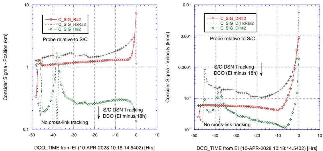
**Figure 3. Baseline Case: Relative position and velocity uncertainty ( $1\text{-}\sigma$ ) of Probe relative to the S/C from probe separation (EI-48h) to EI with no cross-link tracking, but S/C DSN tracking is included. S/C-centered [R,HxR,H] coordinates for the Probe.**
