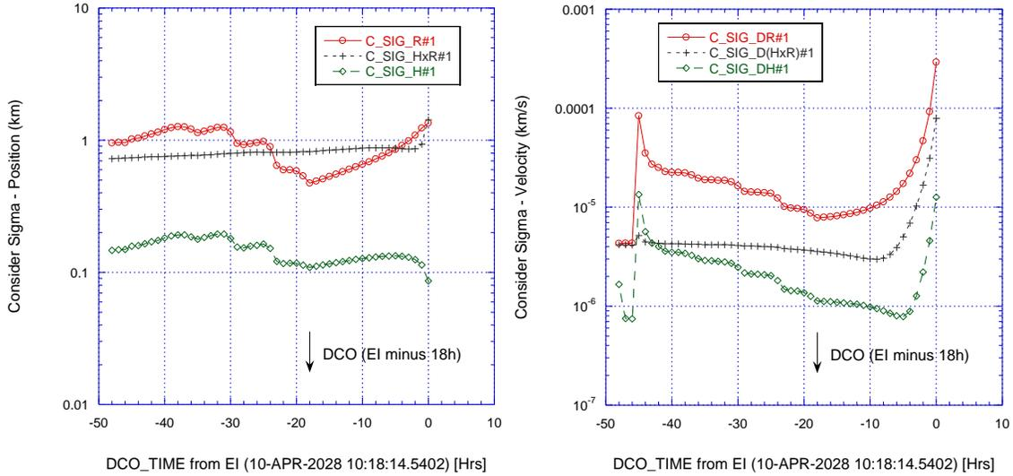
**Figure 1. Baseline Case: Position and velocity uncertainty (1- $\sigma$ ) of S/C from Probe Separation (EI-48h) to EI with DSN tracking only. Venus-centered [R,HxR,H] coordinates.**
