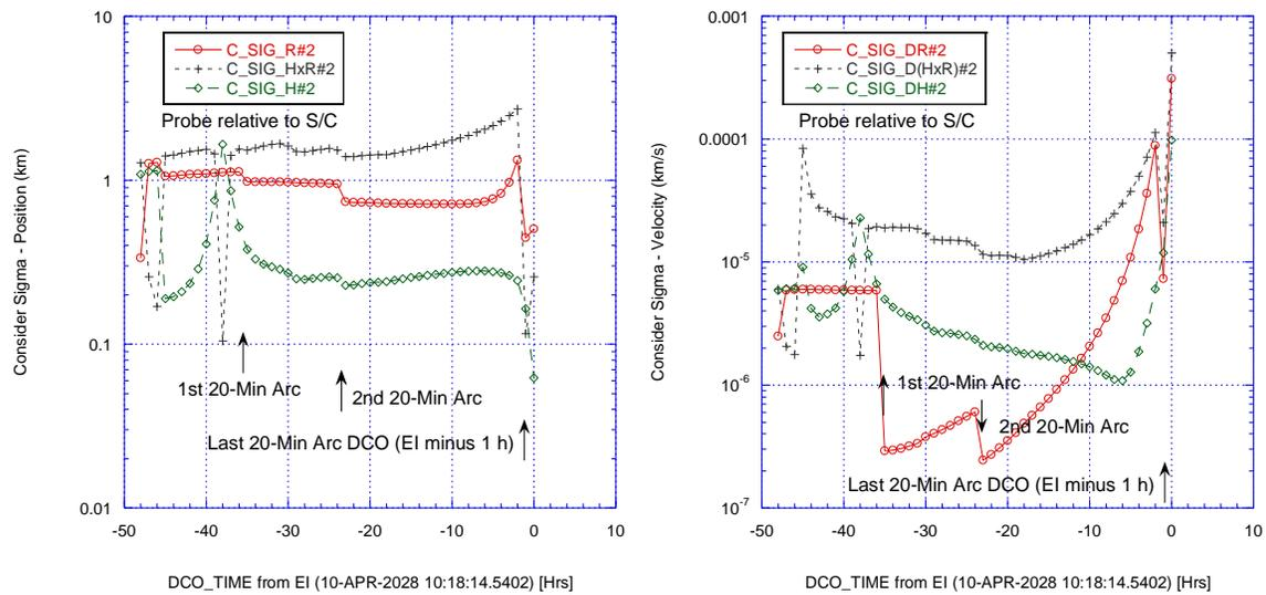
**Figure 5. Relative position and velocity uncertainty (1- $\sigma$ ) of Probe relative to the S/C from probe separation (EI-48 hr) to EI with cross-link Doppler weighted at 1.0 mm/s and S/C DSN tracking. S/C-centered [R,HxR,H] coordinates for the Probe.**
