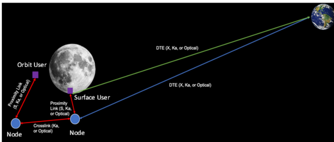
Figure 16 - Functional Interfaces and Corresponding Frequency Bands
