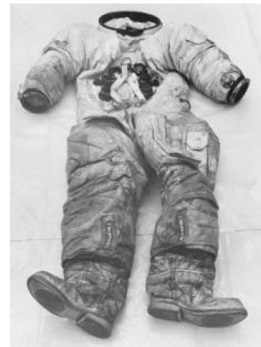
Figure 5. ITMG from model A7L spacesuit worn on the lunar surface by Apollo 12 LMP Alan Bean. Image originally appeared in NASA TR-169-001, prepared at the WSTF.
