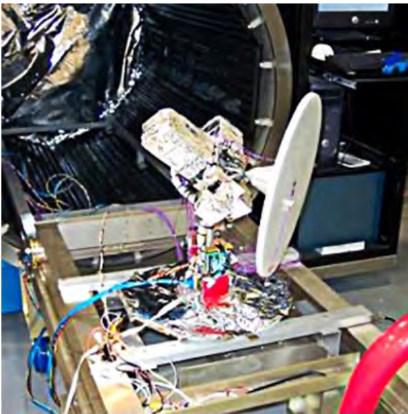
Figure 22. Thermal Vacuum Chamber used for testing Balloon High Gain Antenna (HGA)
