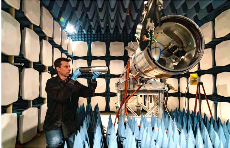
Figure 5: EMI/EMC Measurement Facility
