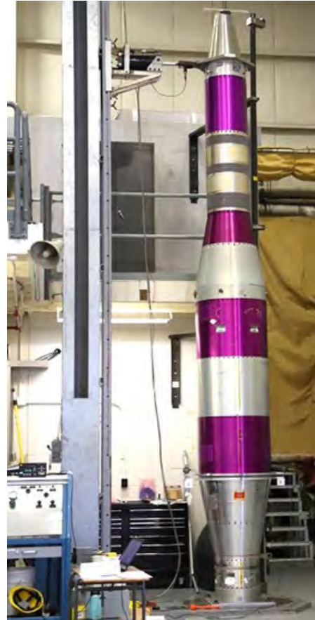
Figure 39: Bend Test Fixture
