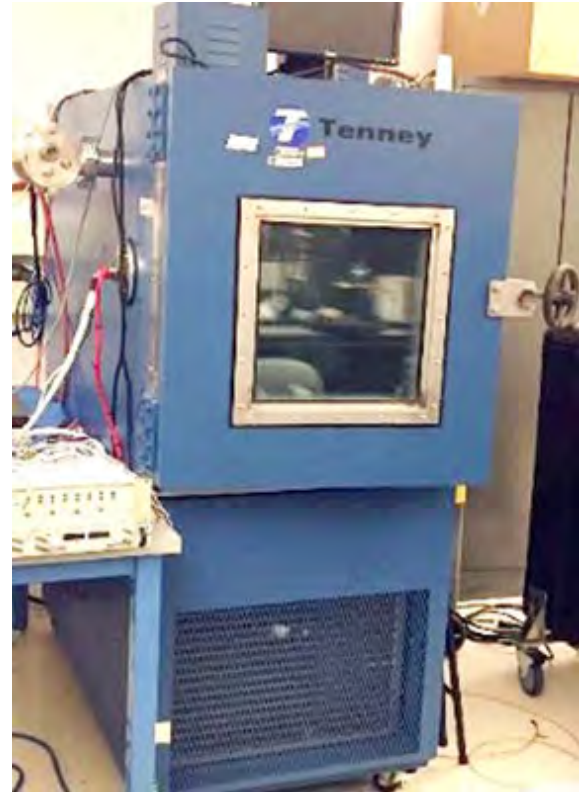
Figure 29: Environmental Test Chamber Model T5ST
