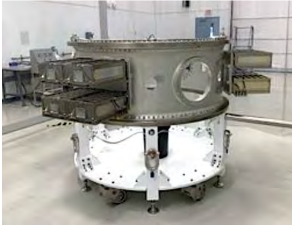
Figure 55: Integrated ESPA ring prior to leaving Wallops (Building F-7)
