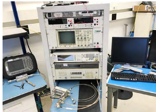
Figure 11: Flight Termination Receiver System Certification Bench
