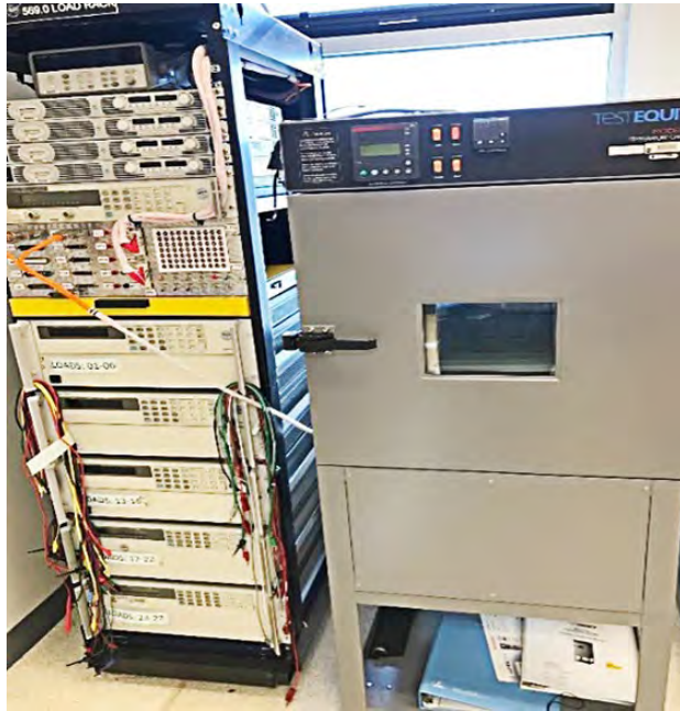
Figure 12: Test Equity Model 115 Thermal Cycle Chamber
