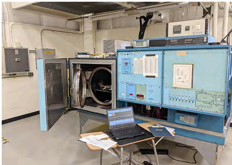
Figure 24. Thermal Vacuum Chamber (Building F-10)
