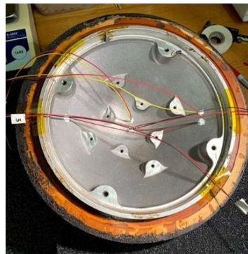
11" capsule with AMTPS heat shield flown by Univ. of Kentucky on NG-16
