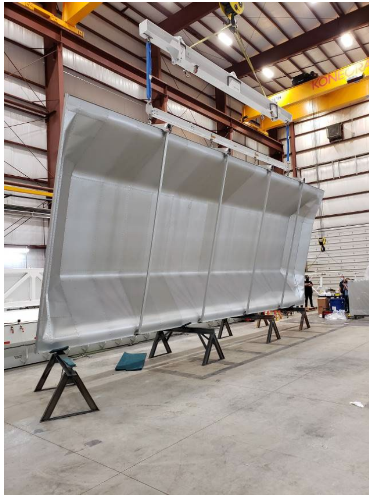
Figure 7. Rotating the lower tent frame for cleaning access ( Credit: NASA/GSFC )
