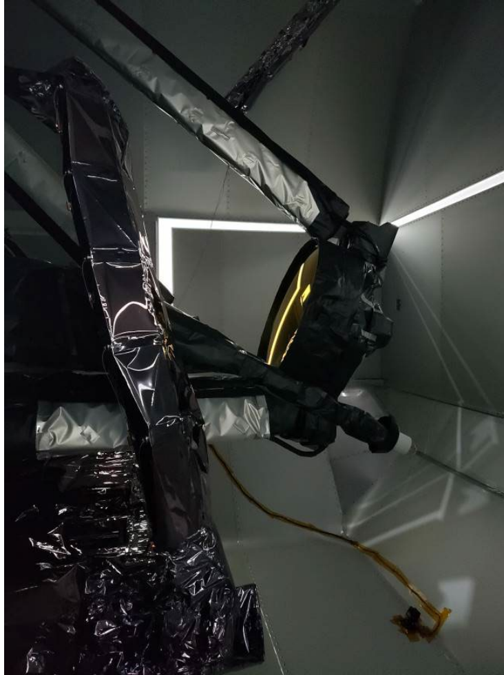
Figure 14. The secondary mirror was the first view of Webb inside OSTTARS at the launch site. (Credit: Joseph Ward)
