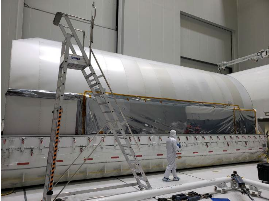
Figure 10. OSTTARS final closeouts around the upper and lower tent frames. (Credit: NASA/GSFC)
