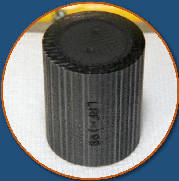
Radioisotope Power System Heat Source
