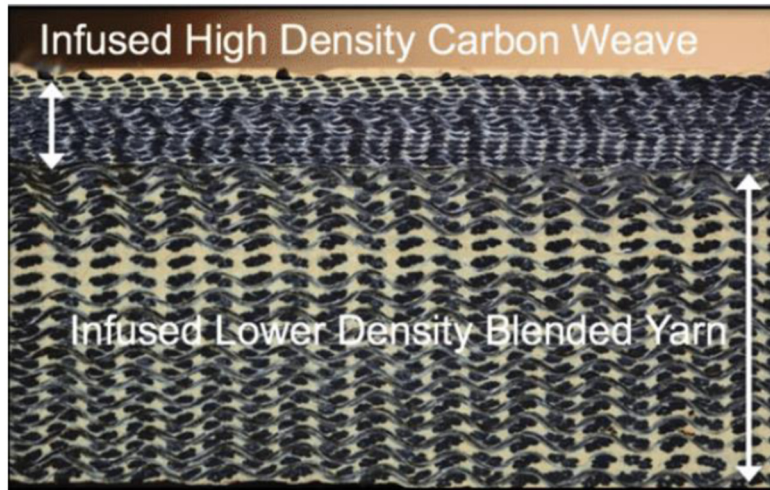
Figure 2. Dual layer 3D woven TPS shown in Fahy et al. [16]. The “Infused Lower Density Blended Yarn” is very similar to the 3D Medium Density Carbon Phenolic (3MDCP) material modeled herein.
