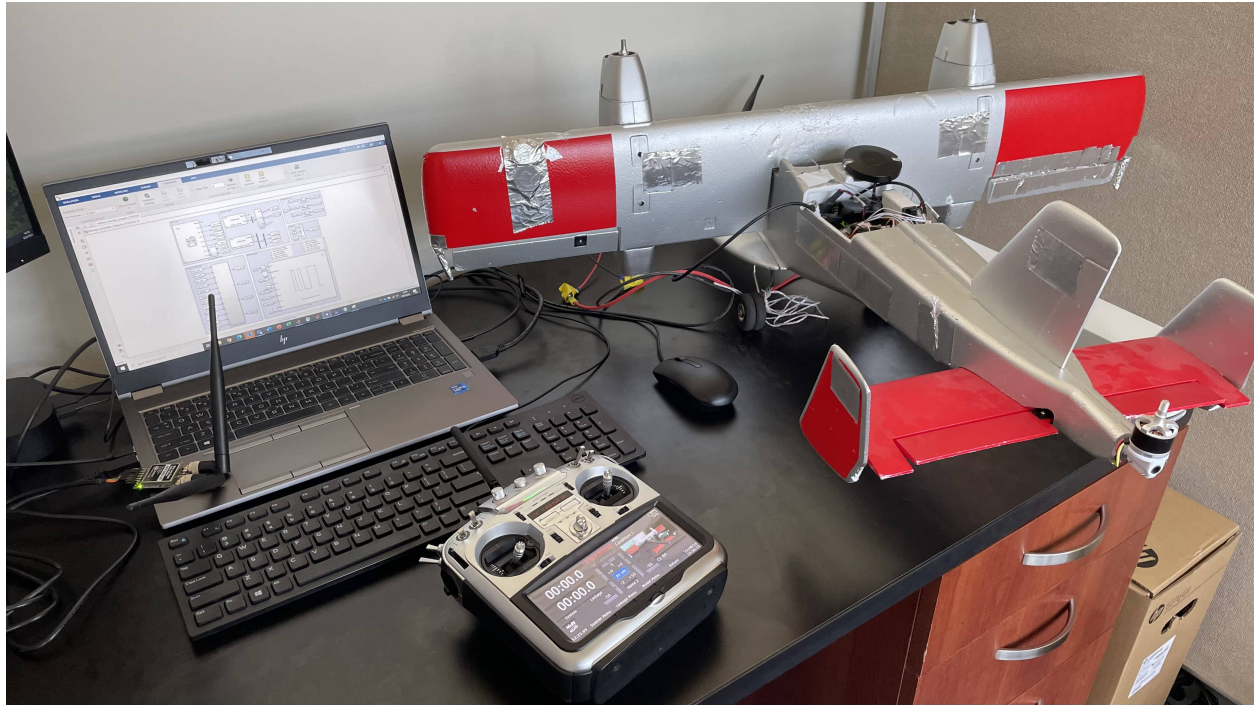
Figure 3: Bench test setup used to run connected simulations.
