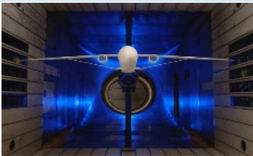
Transonic Truss-Braced Wing 5-10% fuel burn benefit
