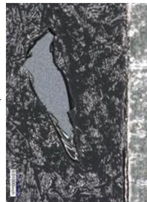
Acrylic "shard" missing after exposure to cryogenic temperatures
