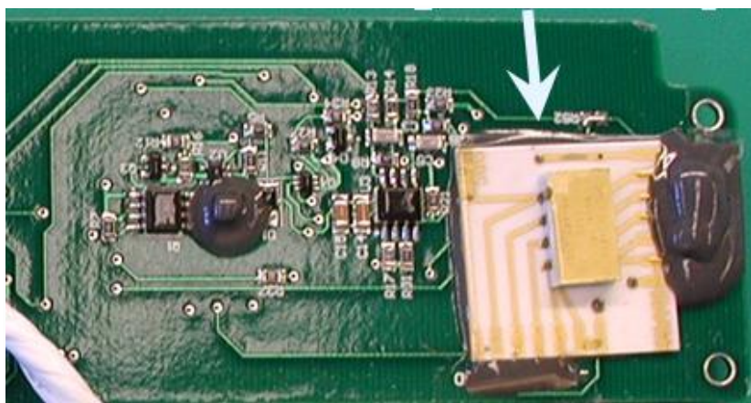
MISSE 7 SiC JFET & Ceramic Packaging (arrow) on a Rad-Hard Electronics Board for ISS flight
