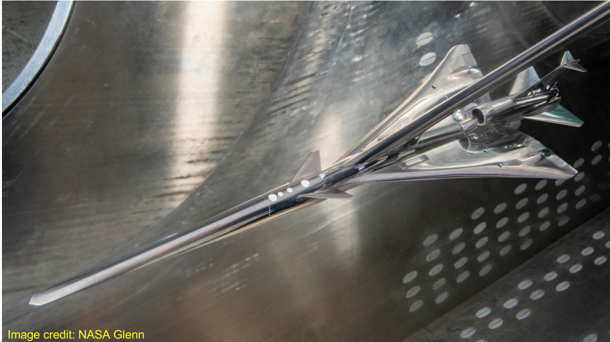
Figure 4-11 Close-up view of upper surface of X-59 model on blade strut in wind tunnel
