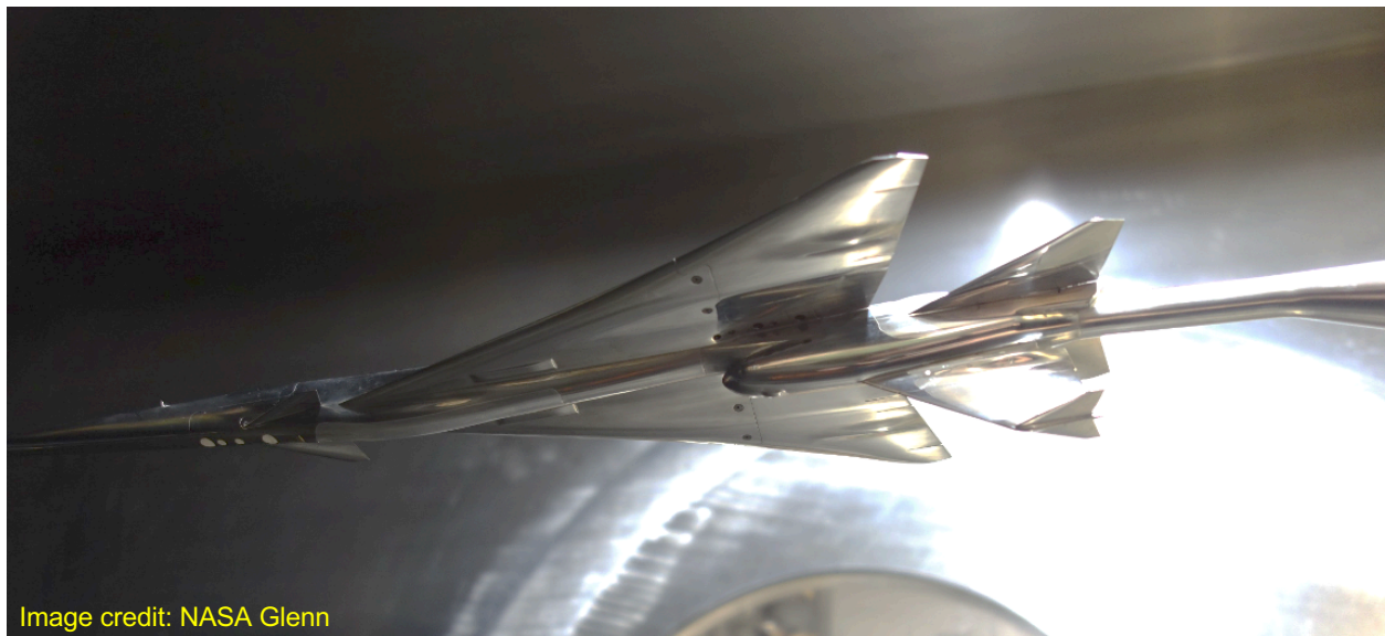
Figure 4-10 View of X-59 model mounted on sting in wind tunnel
