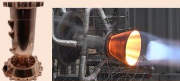
**NASA HR-1**, high strength superalloy for hydrogen environments
