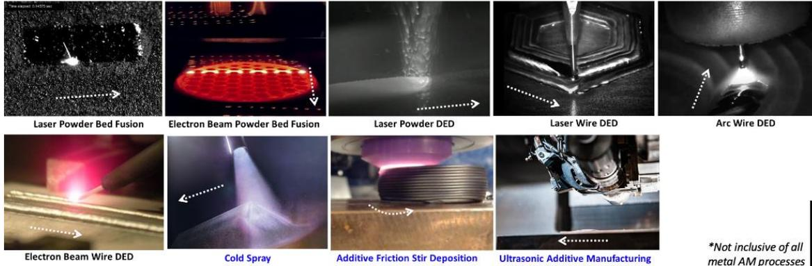
A) Laser Powder Bed Fusion [https://doi.org/10.1016/j.actamat.2017.09.051], B) Electron Beam Powder Bed Fusion [Credit: Courtesy of *Freemelt AB*, Sweden], C) Laser Powder DED [Credit: *Formalloy*], D) Laser Wire DED [Credit: *Ramlab* and *Cavitar*], E) Arc Wire DED [Credit: *Institut Maupertuis* and *Cavitar*], F) Electron Beam DED [NASA], G) Cold spray [Credit: *LLNL*], H) Additive Friction Stir Deposition [NASA], I) Ultrasonic AM [Credit: *Fabrisonic*].
