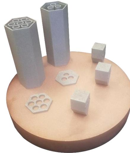
First NASA W AM build: NTP fuel clad with integrated coolant channels.
