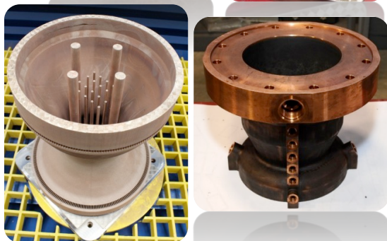
GRCop-84 3D printing process developed at NASA and infused into industry
