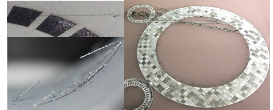
Locked Build Files: Stray vectors Created During Re-slicing
