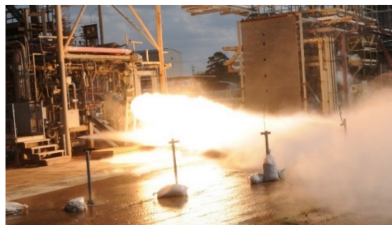
Ox-Rich Staged Combustion Subscale Main Injector Testing of 3D-Printed Faceplate
