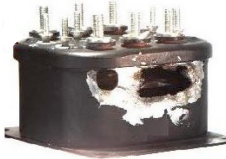
Failed relay due to tin vapor arcing
