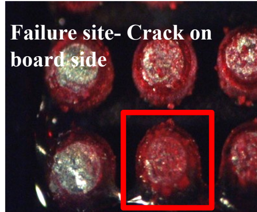
(a) Failure on board side
