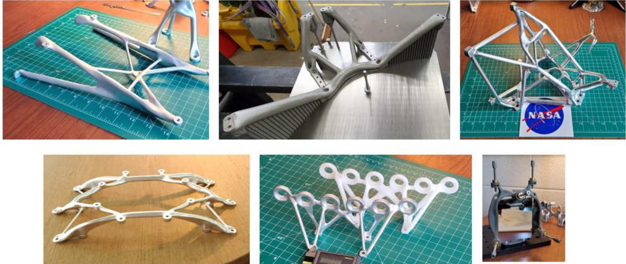
Figure 6. Other applications of the Evolved Structures process include the EXCITE radiator bracket (top left), the EXCITE cryostat mount (top center), the ALICE Optical Bench (top right), the STAR-X detector mount (bottom left), the CCRS diode bracket (bottom center), and the NGXO mirror mount (bottom right).
